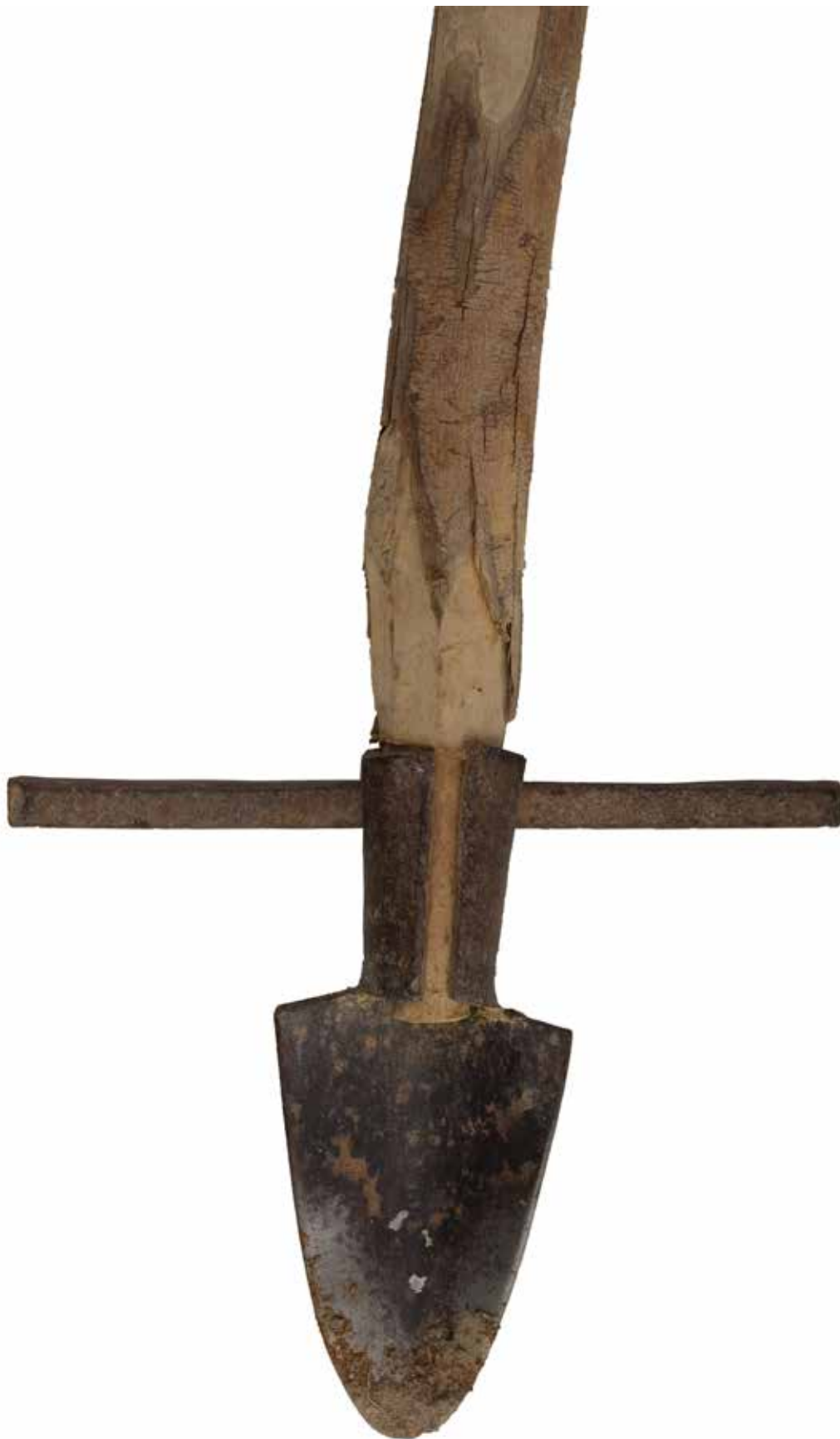
Figure 23: Spade with a handle consisting of a long wooden stick with some of the bark still present. The small triangular blade has a socket that enables it to be attached to the handle. A metal bar with a triangular cross-section has been welded to the top of the socket, creating two foot rests. Length triangular bar: 22 cm (Taşköprü, Turkey; August 2015; RC).
