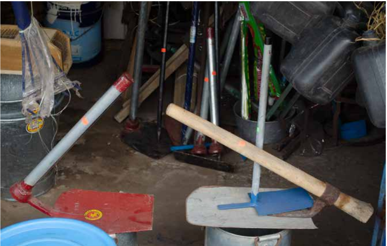
Figure 24: New and second-hand pull hoes offered for sale. The handle is secured either perpendicular to the blade or obliquely to the blade. The hoes also differ in the absence or presence of a stem between the blade and the handle (Kochin, India; January 2015; RC).
