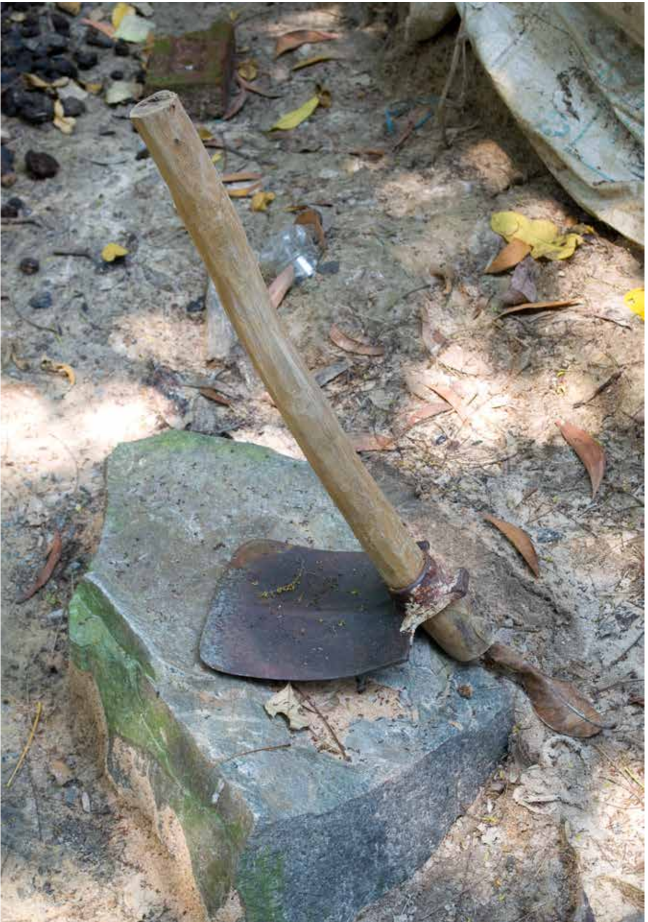
Figure 26: Stemless pull hoe with a slightly curved blade, resting on a stone in the courtyard of a farmhouse. The handle is inserted into the blade (Jaypur, India; September 2014; RC).
